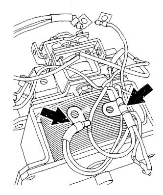
Checking pull-in winding
